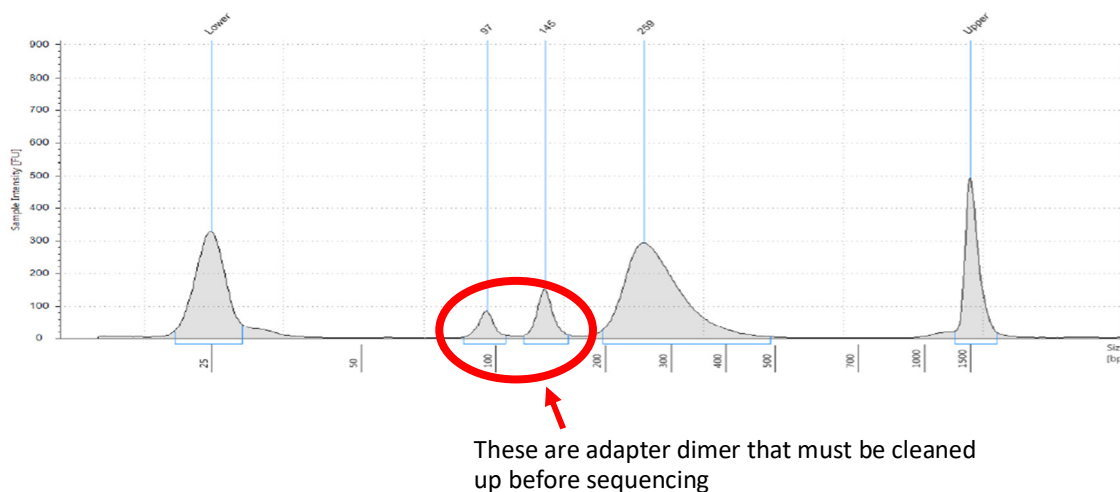
Figure 4 Example of a bad library on a D1000 tape assay on the TapeStation. The peaks between 90– 150 bp (circled) indicates the presence of either primer dimers or excess indexes.
