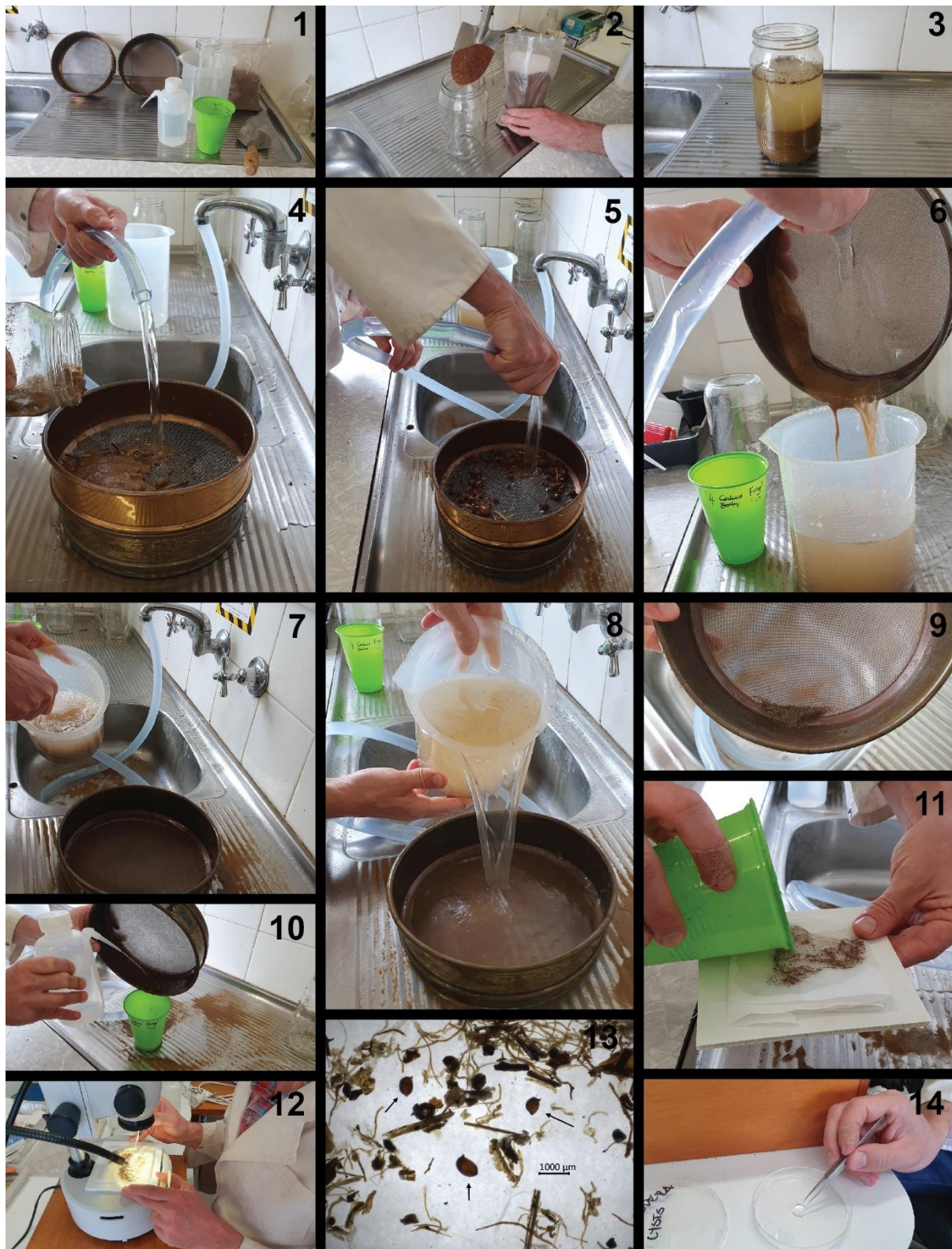
Figure 4. Pictorial guide to Cobb's Sieving and Decanting method (Cobb, 1918); Steps described in section 3.3.2. Images by Manda Khudhir & Daniel C. Huston, CSIRO.
