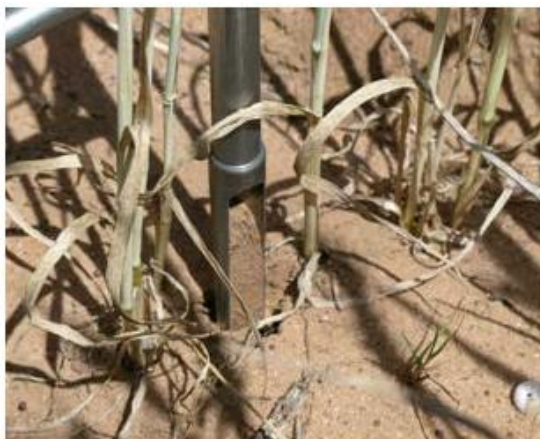
Figure 3. Soil corer being used to take soil samples in vicinity of crop.
