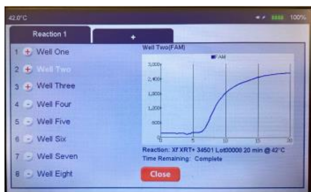
Figure S9.6. Example test results displayed next to the well designation on the screen of an AmpliFire instrument. Results are interpreted as ( + ) = Positive for Xf ( - ) = Xf not detected ( ! ) = Invalid
